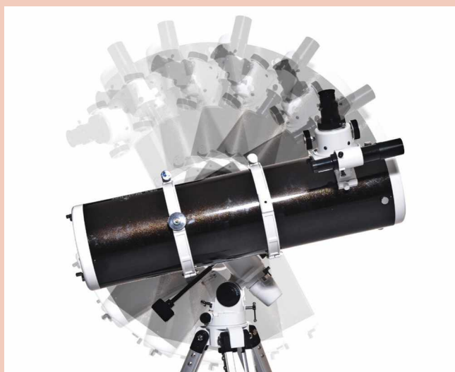
▲ On an equatorial mount, adjust the declination (dec.) axis to move your telescope in a north-south direction...
